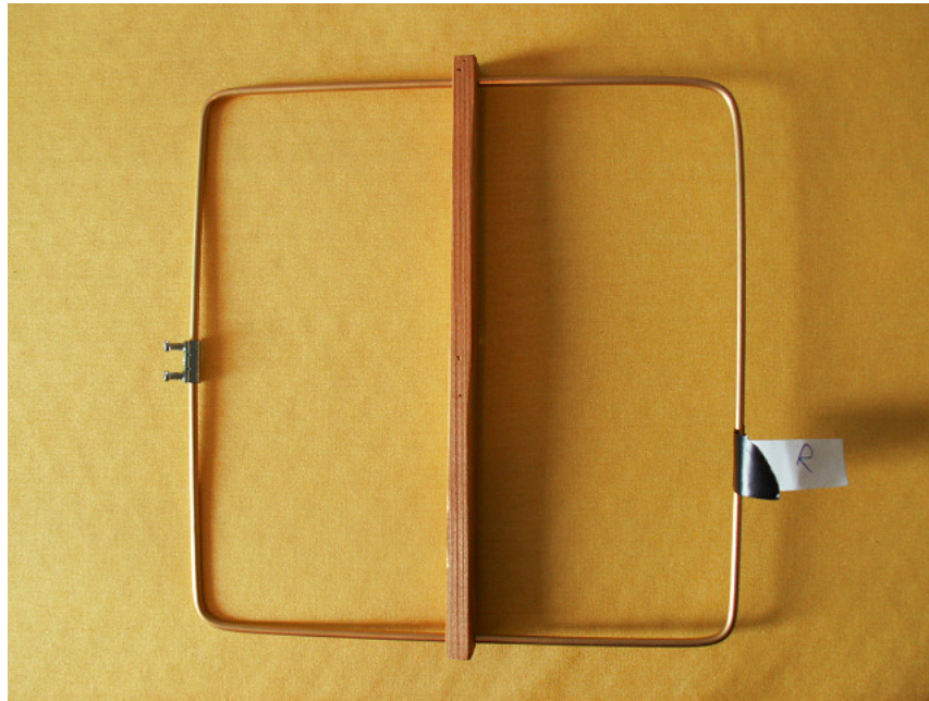
4. picture – The reflector element (beta version, a little bit asymmetric)
