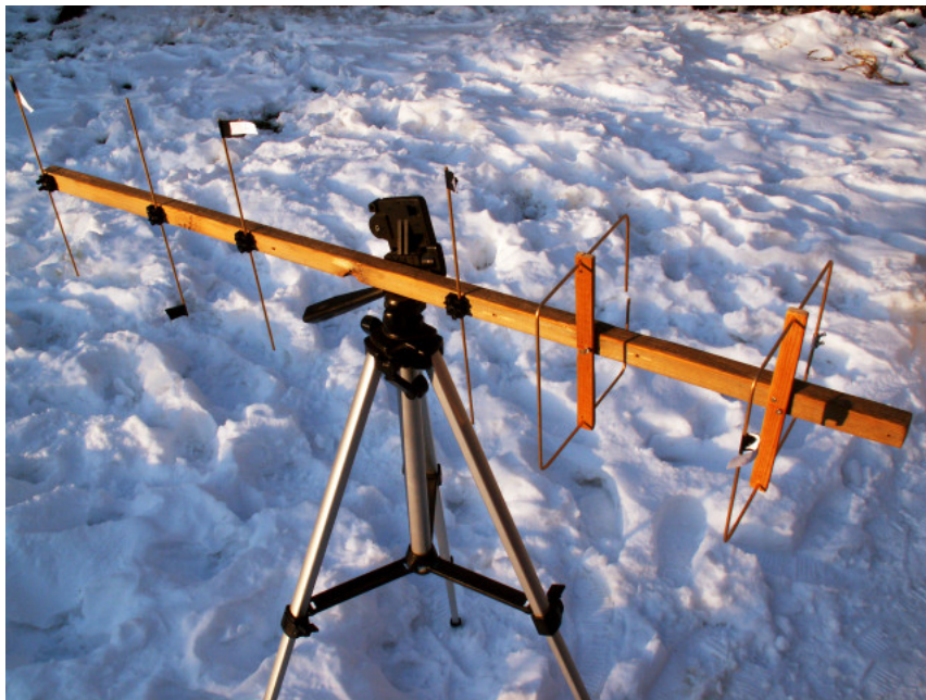
5. picture – The completed quagi, ready for the tuning procedure
